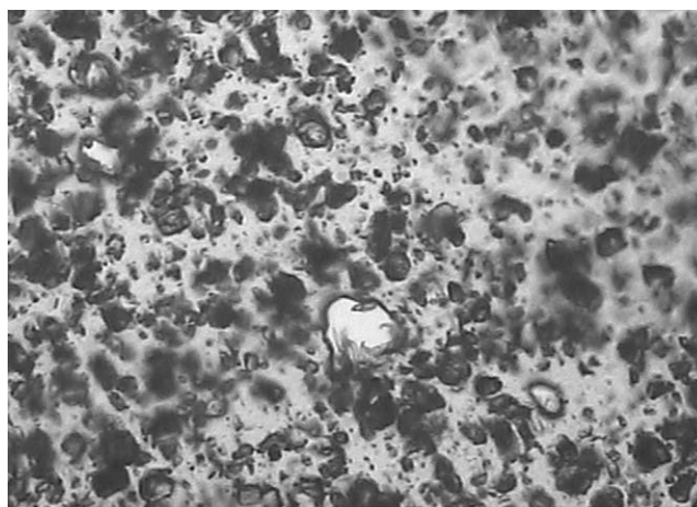
Figure 15. POM image of the ultrathin section from PP/EADP30 (200 \times ).
